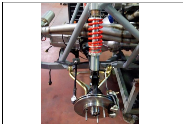
7AM) Suspension arrière montée Rear mounted suspension
