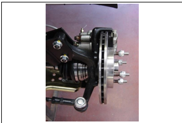
7AL) Suspension arrière montée Rear mounted suspension
