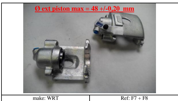
8G) Étrier version standard Rear caliper standard version
